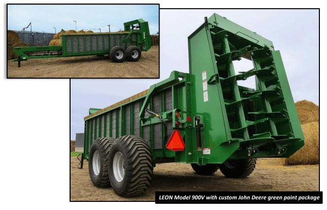
Yorkton, SK – November 1st - LEON'S MFG. COMPANY INC. proudly offers the LEON Model 900 Vertical Hydra Push Spreader. The Model 900V boasts a carrying capacity of 1152 cu. ft. or 926 bushels and delivers a finer, wider and more consistent spread pattern of over 40 feet (12 meters). Custom Color Packages available.
