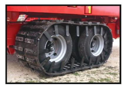
Right Tracks available for a variety of agriculture machinery including: sprayers, trailers, tractors, irrigation pivots, etc.
