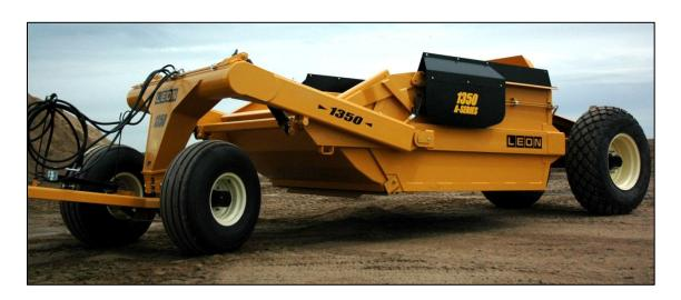
Yorkton, SK - June, 2011 - NEW for 2011, LEON'S MFG. COMPANY INC. proudly offers the NEW LEON MODEL 1350 A-SERIES Land Scraper. Designed for agricultural and industrial applications, the large 13.5 cubic yard capacity unit features HD Twin RAM Cylinder forced ejection capabilities, rear diamond back construction tires, fully synchronized hydraulic control, and 180 deg ++ ball and socket steering for maximum manoeuvrability.
