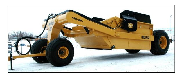
**Yorkton, SK – Feb, 2011 -** NEW for 2011, LEON'S MFG. COMPANY INC. proudly offers the NEW LEON MODEL 2050 I-SERIES Land Scraper. Designed for agricultural and industrial applications, the extra large 20.5 cubic yard capacity unit features HD Twin RAM Cylinder forced ejection capabilities, rear diamond back construction tires, fully synchronized hydraulic control, and 180 deg ++ ball and socket steering for maximum manoeuvrability.
