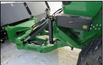
LEON Dozer Blade mounting design ensures full tractor accessibility and serviceability while taking special care not to interfere with tractor engine panels, tractor hoods, and tractor lights.
