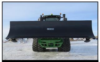
Superior LEON Blade Lift Height for packing, stacking, pushing and piling. LEON also features the industry's highest blade under clearance which is ideal for working in soft, uneven terrain.
