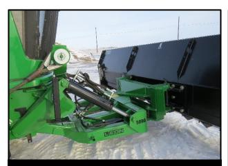
LEON's patented 'Quick On-Quick Off' mounting system features custom color push frame, winch cable hook guard, parking stands, plus quick disconnect couplers as standard equipment.
