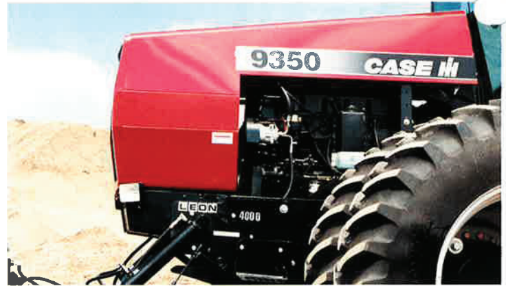
Full side panel access for tractor servicing
