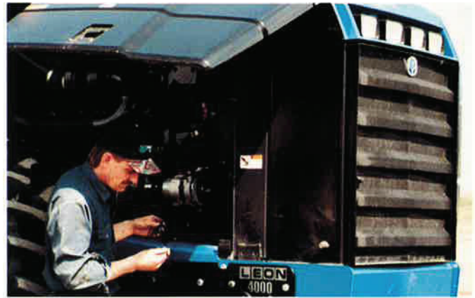
Full side panel access for tractor servicing
