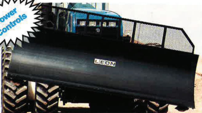
Power Tilt & Angle is an extra feature that has become a necessity for this heavy duty equipment. Invest initially or add on to the same unit at a later date. The cylinders are positioned to avoid contact with material being dozed.
