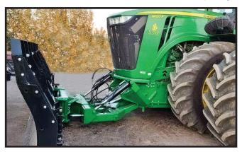
Powerful 'industrial strength' RAM Hydraulic Cylinders are strategically positioned on LEON Dozer systems to avoid exposure to debris when in operation.
