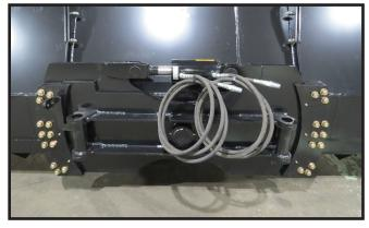
Hydraulic 6 Way Vertical Tilt can be instrumental when shaping land and roads. This valuable accessory can be added to any LEON 2WD, 4WD, or Track Drive Dozer Blade at time of order or down the road.
