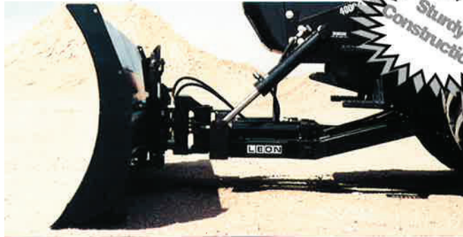
Sturdy Construction and Mounting is featured to insure these units stand up in the toughest of conditions. Push pressure is transmitted from the front tractor section & is designed to place minimum stress on the tractor framework. All hydraulics included.
