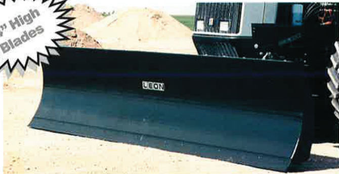
New High Definition 440 Blades are 44" (112 cm) high in 10 ft. (3.05 m) to 16 ft. (4.88 m) widths. The ripple formed blade insures clean roll off and roll break action to make pushing easier for the tractor.
