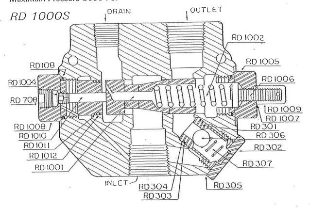
Internal pilot and external drain
